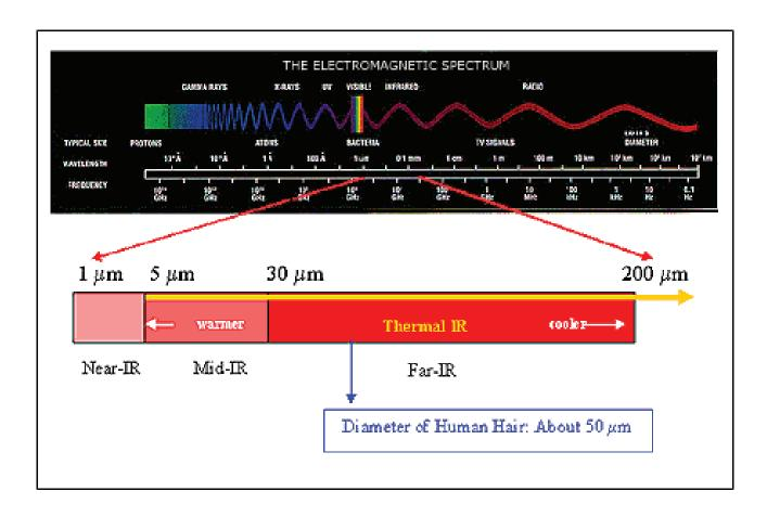
Astronomers often refer to different types of infrared light, although the precise wavelength ranges are somewhat arbitrary. For the most part, infrared light is thermal radiation; that is, it is a measure of heat. Cooler objects emit IR light at longer wavelengths.
